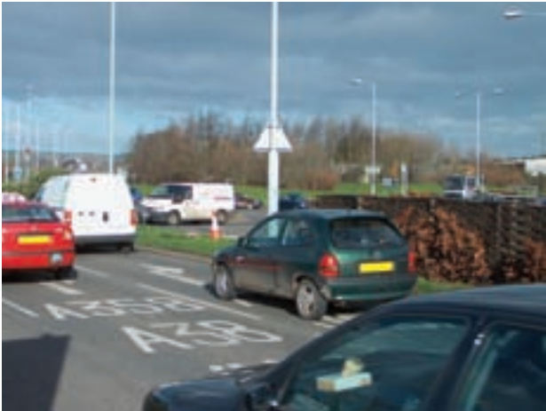
Figure 9.10 Visibility to the right reduced by sight screens (Alex Sully)
