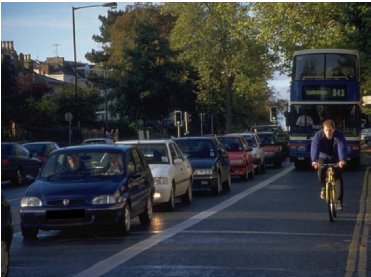
Figure 6.1 Narrow 3-metres wide bus lane (Sustrans)
